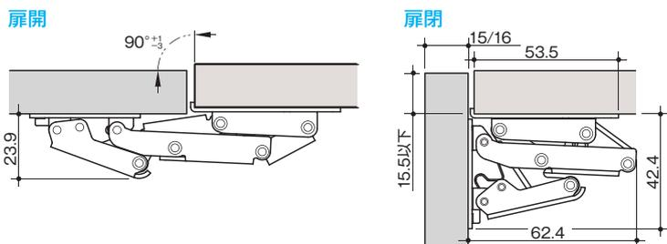
Hinge for wood thickness of 16mm
